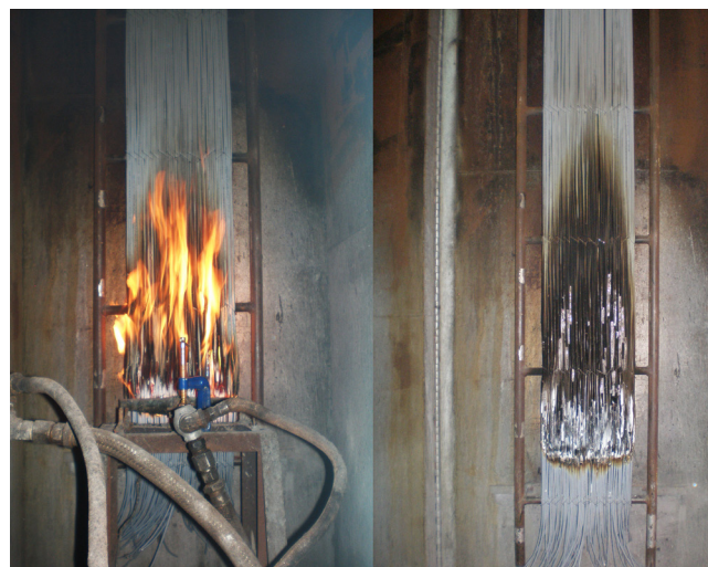
Full scale fire test to EN50575
